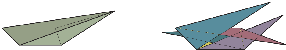
FIGURE 3. An impossible configuration of four collapsing walls (sides of a pyramid cannot collapse on the base and leave an uncovered hole in the base).
